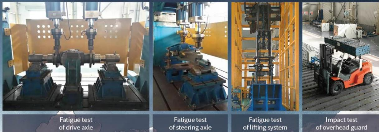
Fatigue test of drive axle
