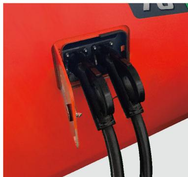
Lithium battery forklift truck is equipped with double gun charging as standard, which greatly reduces the charging time. Lithium batteries have high-density capability and can be used and charged at any time to realize efficient and continuous operation all day long.
